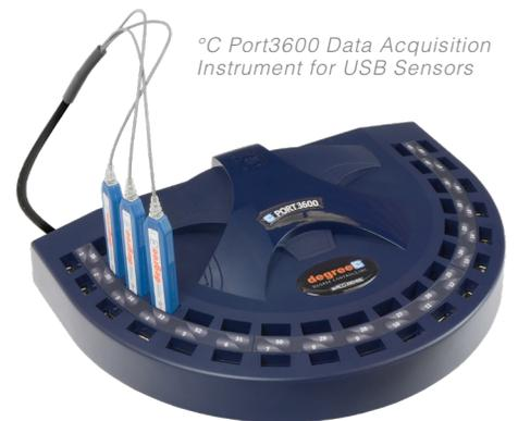
°C Port3600 Data Acquisition Instrument for USB Sensors
