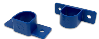
°C Clamp End Mount (left) or Side Mount (right) - Perpendicular or parallel to sensor - #10 screw fits thru holes
