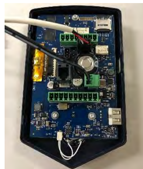
Figure 16 Power & Sensor Connection
