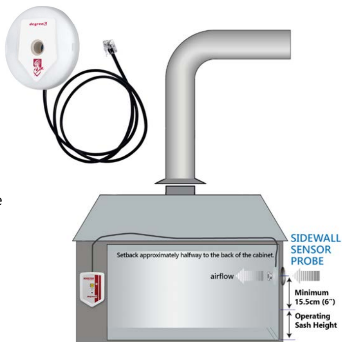
Figure 5 Align Sensor Head Into Direction of Airflow
