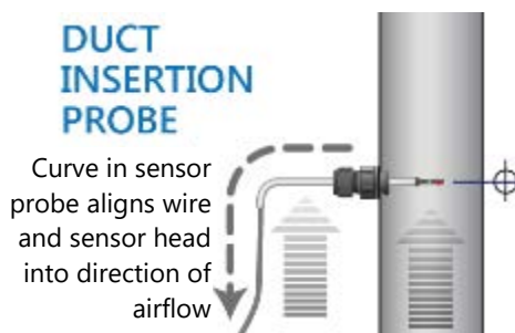
Figure 5 Align Sensor Head Into Direction of Airflow
