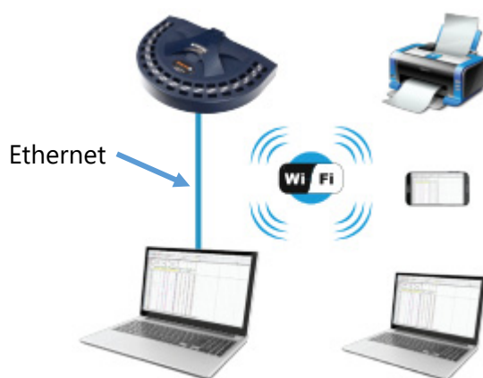
Figure 15 Ethernet - Direct to PC with Static IP Addressing Dedicated PC Connection
