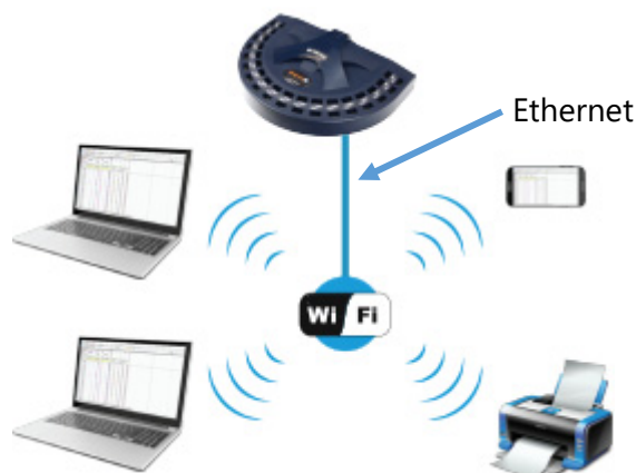
Figure 14 Ethernet - °C Port to Network with Dynamic IP Addressing Direct Router Connection
