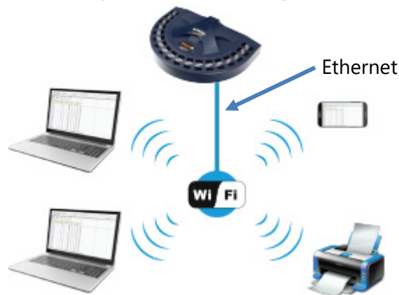
Figure 8 Ethernet - °C Port to Network with Dynamic IP Addressing Direct Router Connection
